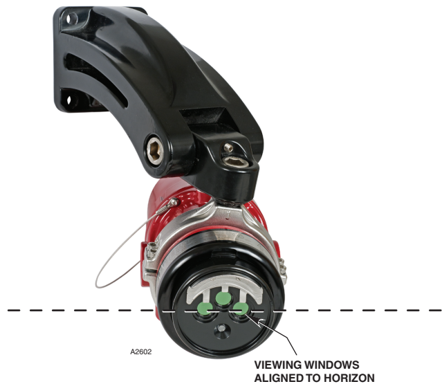
Figure 8—Optimal Alignment of Viewing Windows (X3301 with Collar Attachment)
